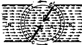
FIG. 205.—ACTIVE CONDUCTOR LEAVING POLAR FLUX.
